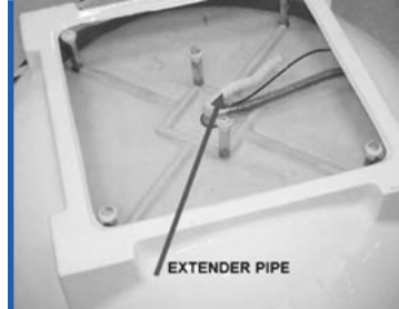
Picture 3: The waste-overflow fitting is pre-installed with the bathtub at the factory. The corrugated extender must be removed and discarded unless there is absolutely no other way to complete the installation. The waste pipe/p-trap connection must be made directly to waste/drain outlet located at the bottom of the tub.
